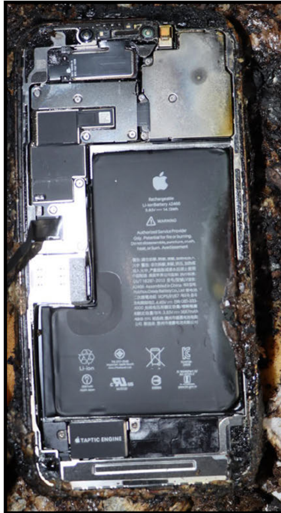
Photograph of subject iPhone and ruptured battery at incident location (above)
