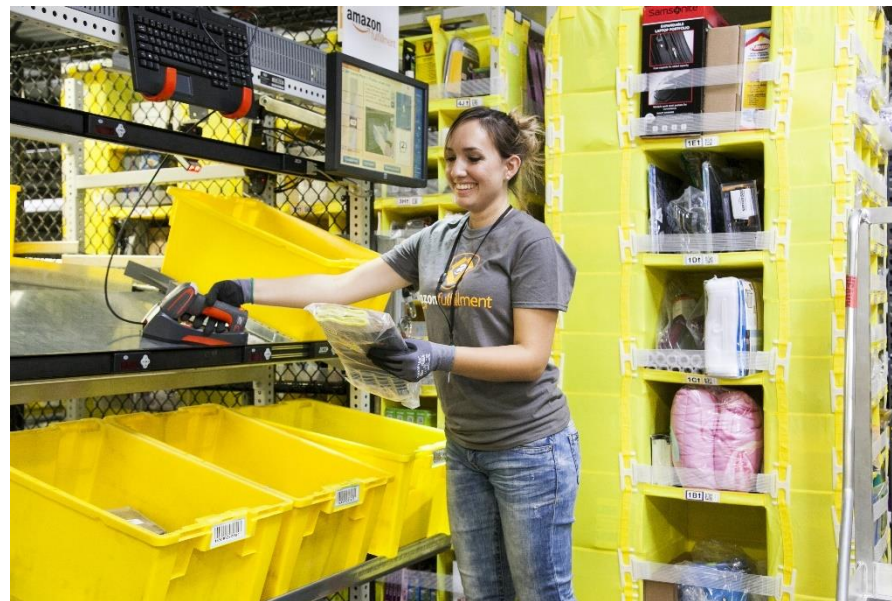
Fig. 5. Female picker scanning item picked from pod to place in tote on rack at workstation. 5
